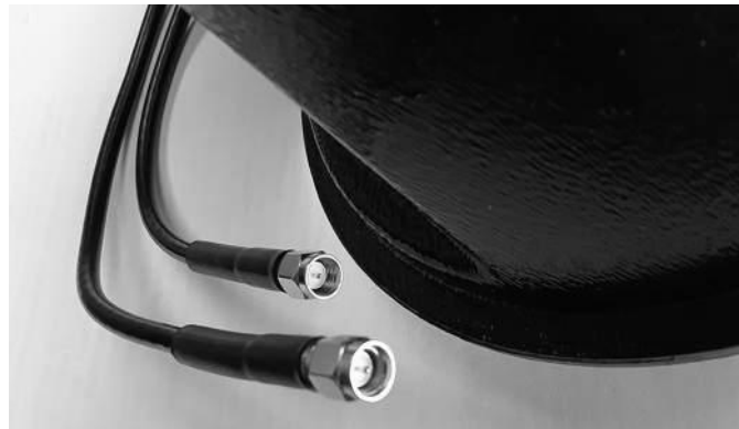
Figure 24. Cradlepoint Antenna Connector Pins
