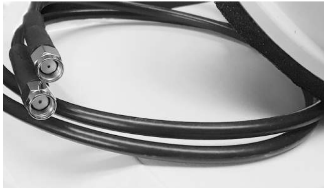
Figure 23. Moxa Antenna Connections Have Female Pins
